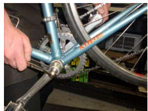
Jeremy having way too much fun installing a new bottom bracket into a 25 year old Rodriguez bicycle. This bike looks great, and was back on the road a day or 2 after the customer brought it in for service. Thanks to the ISO commission of the 1970's, this bicycle will probably be on the road another 50 years or more.
